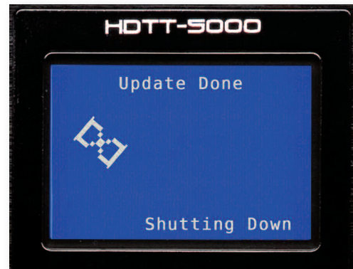
Fig 3.3 - Power shuts off completely when the update is complete
